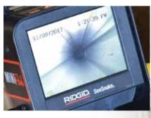
Daviesway DASCO's Shaun Kingston can check the entire milk line within minutes with an inline camera.
